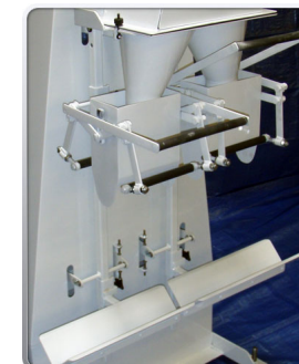
Easy to use twin grip bag clamps and adjustable height sack supports.
