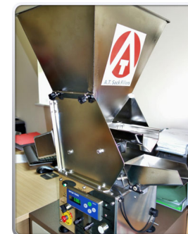
Pneumatic operated tipping weigh pan.
