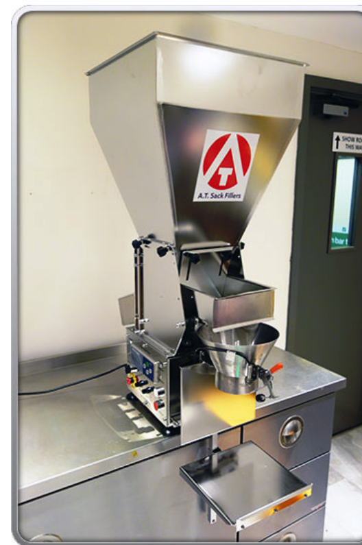
Pneumatic operated tipping weigh pan.
