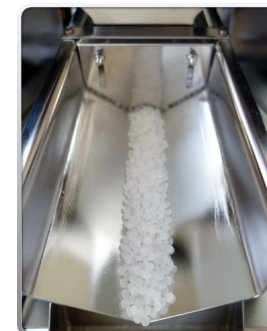
V design feeders for more controlled and accurate product delivery.
